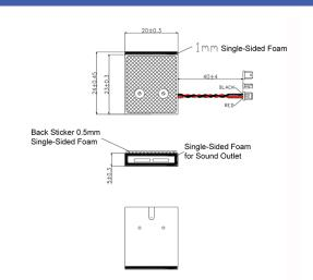
General tolerance = ±0.3 mm and all measurements in mm unless otherwise noted
