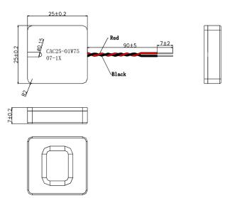
General tolerance = ±0.2 mm and all measurements in mm unless otherwise noted.
