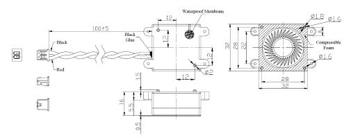
General tolerance = ±≤2 mm: ±0.1 mm, >2 mm: ±0.3 mm and all measurements in mm unless otherwise noted.
