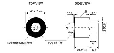
General tolerance = ±0.5 mm and all measurements in mm unless otherwise noted.
