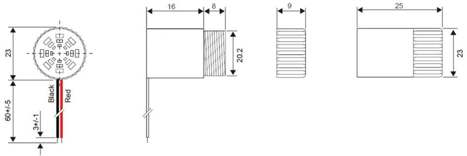
General tolerance = ±0.5 mm and all measurements in mm unless otherwise noted.
