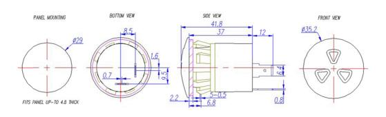
General tolerance =  $\pm 0.75$  mm and all measurements in mm unless otherwise noted.
