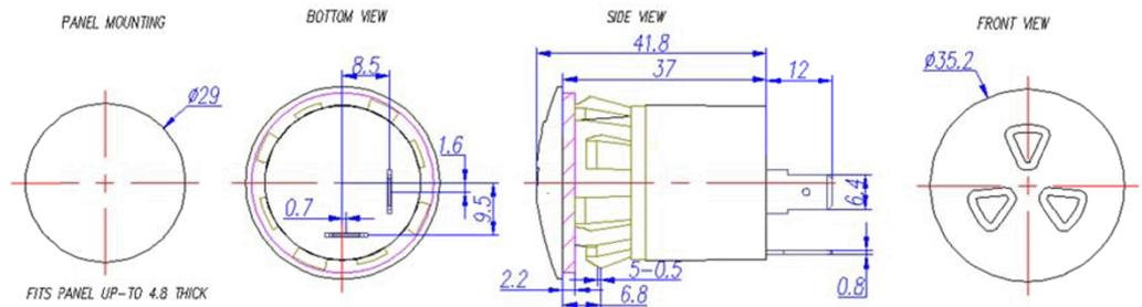
General tolerance =  $\pm 0.75$  mm and all measurements in mm unless otherwise noted.
