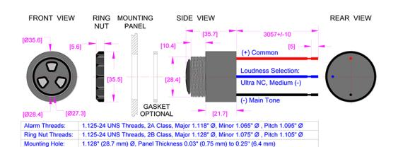
Rubber, ID 1.18" (30.0 mm), OD 1.40" (35.6 mm), Thickness 0.10" (2.54 mm)
