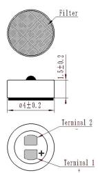
General tolerance =  $\pm 0.2$  mm and all measurements in mm unless otherwise noted.
