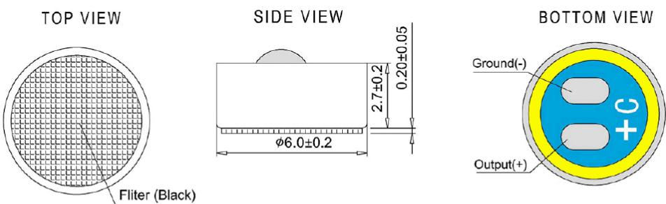
General tolerance = ±0.1 mm and all measurements in mm unless otherwise noted.
