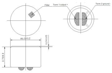
General tolerance =  $\pm 0.2$  mm and all measurements in mm unless otherwise noted.
