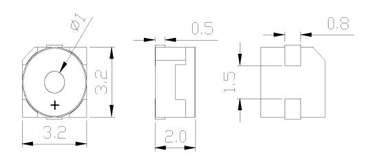
General tolerance = ±0.3 mm and all measurements in mm unless otherwise noted.
