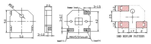
Unless otherwise specified, tolerance:  $\pm 0.5$  (unit: mm)
