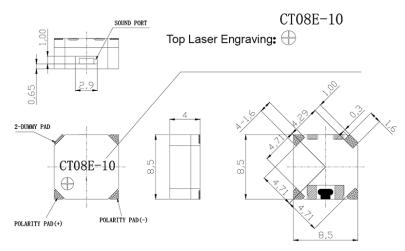
General tolerance =  $\pm 0.5$  mm and all measurements in mm unless otherwise noted.
