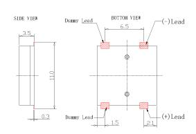
General tolerance = ±0.5 mm and all measurements in mm unless otherwise noted.
