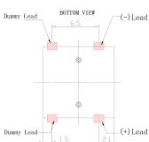
General tolerance =  $\pm 0.5$  mm and all measurements in mm unless otherwise noted.
