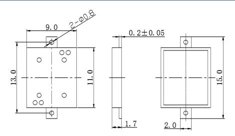
General tolerance = ±0.5 mm and all measurements in mm unless otherwise noted.
