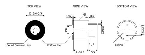
General tolerance = ±0.5 mm and all measurements in mm unless otherwise noted.
