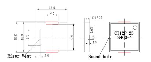
General tolerance =  $\pm 0.5$  mm and all measurements in mm unless otherwise noted.
