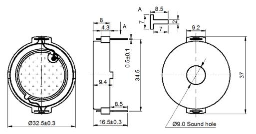
General tolerance = ±0.5 mm and all measurements in mm unless otherwise noted.
