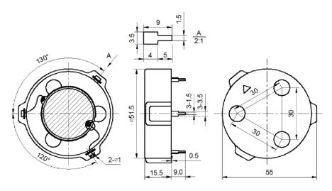
General tolerance =  $\pm 0.5$  mm and all measurements in mm unless otherwise noted.
