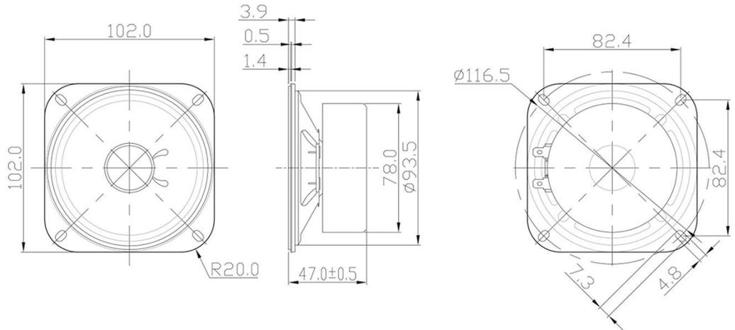
General tolerance = ±0.3 mm and all measurements in mm unless otherwise noted.
