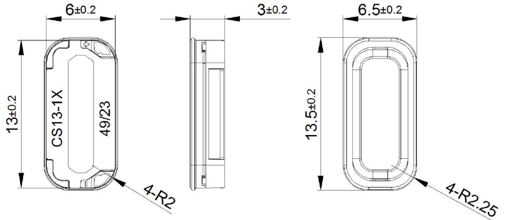
General tolerance =  $\pm 0.5$  mm and all measurements in mm unless otherwise noted.
