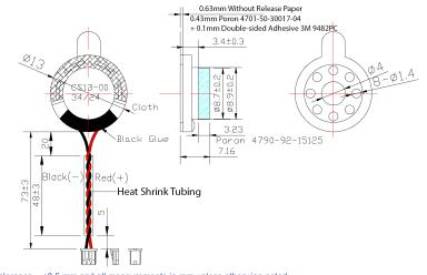
General tolerance =  $\pm 0.5$  mm and all measurements in mm unless otherwise noted.
