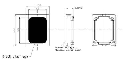
General tolerance =  $\pm 0.2$  mm and all measurements in mm unless otherwise noted.
