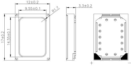
General tolerance =  $\pm 0.2$  mm and all measurements in mm unless otherwise noted.
