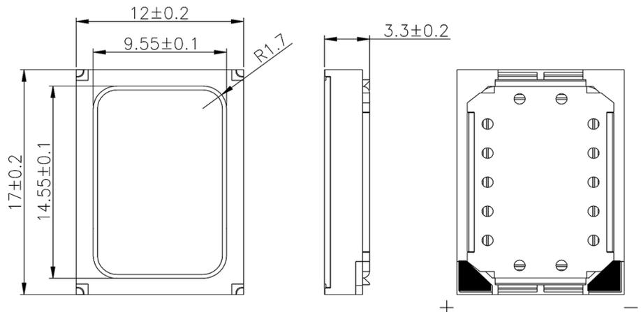
General tolerance = ±0.2 mm and all measurements in mm unless otherwise noted.
