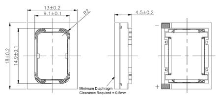
General tolerance =  $\pm 0.2$  mm and all measurements in mm unless otherwise noted.
