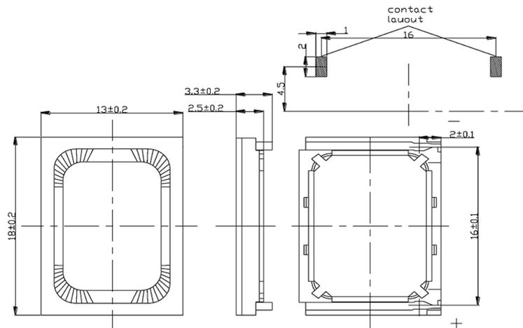
General tolerance = ±0.2 mm and all measurements in mm unless otherwise noted.
