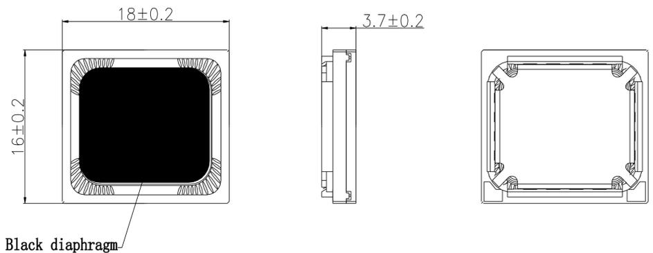
General tolerance = ±0.2 mm and all measurements in mm unless otherwise noted.
