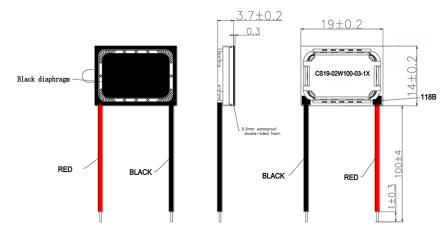
General tolerance =  $\pm 0.2$  mm and all measurements in mm unless otherwise noted.
