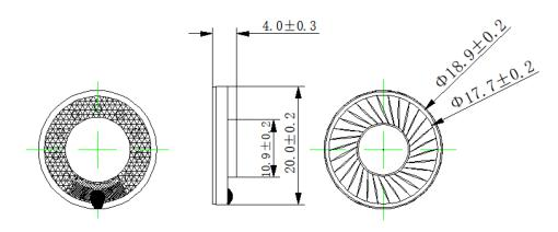
General tolerance = ±0.2 mm and all measurements in mm unless otherwise noted.
