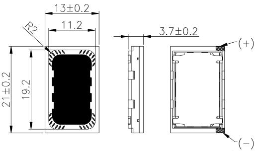
General tolerance = ±0.2 mm and all measurements in mm unless otherwise noted.
