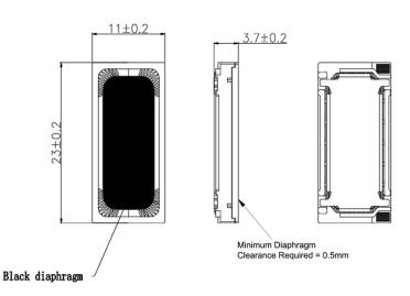
General tolerance = ±0.2 mm and all measurements in mm unless otherwise noted.
