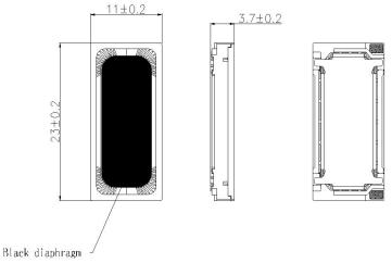
General tolerance =  $\pm 0.2$  mm and all measurements in mm unless otherwise noted.
