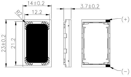
General tolerance = ±0.2 mm and all measurements in mm unless otherwise noted.
