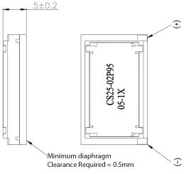
General tolerance =  $\pm 0.2$  mm and all measurements in mm unless otherwise noted
