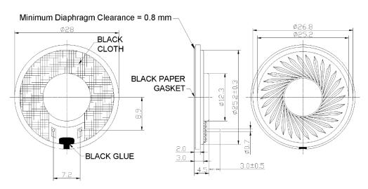
General tolerance =  $\pm 0.5$  mm and all measurements in mm unless otherwise noted.
