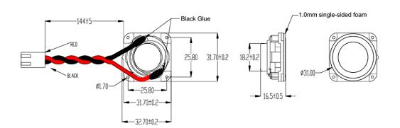
General tolerance =  $\pm 0.5$  mm and all measurements in mm unless otherwise noted.
