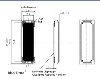
General tolerance =  $\pm 0.2$  mm and all measurements in mm unless otherwise noted.
